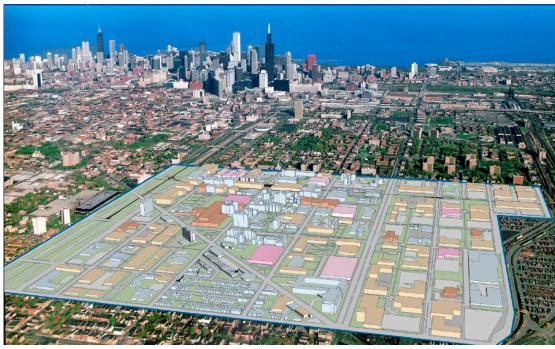
hood streets to create internal through-block pedestrian connections. At the same time, density in the District was reassessed. It was determined that the average FAR was unrealistically high in relation to the proposed street layout and development potential, and therefore was reduced. The resulting Master Plan is a series of internal and individual campuses with buildings fronting onto central park spaces.
