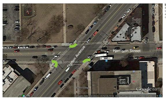
Image: Bump outs, or tightened turn radii are needed on diagonal streets
